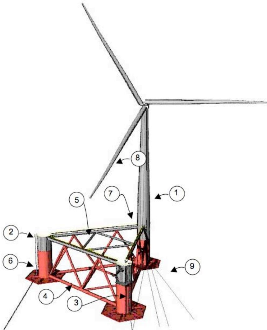
**Figure 1-6** - WindFloat integrated with 5MW turbine
